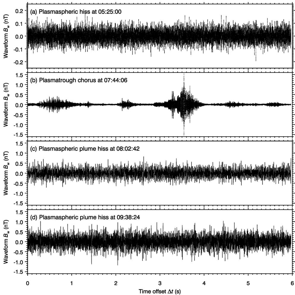
**Figure 2.** Waveform bursts of (a) plasmaspheric hiss, (b) plasmatrough chorus, and (c, d) plasmaspheric plume hiss detected by RBSP-B.
