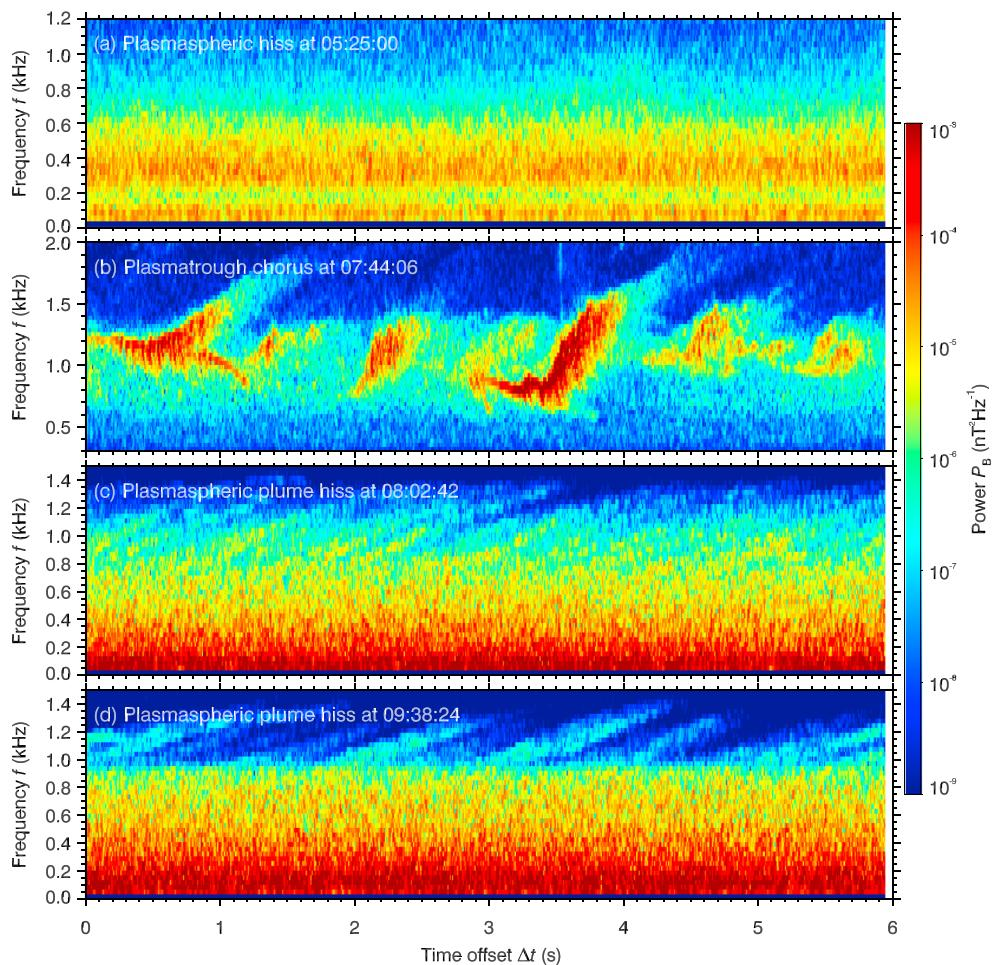
**Figure 5.** Burst frequency-time spectra of (a) plasmaspheric hiss, (b) plasmatrough chorus, and (c, d) plasmaspheric plume hiss detected by RBSP-B. The covered time periods are exactly same as those in Figure 2.
