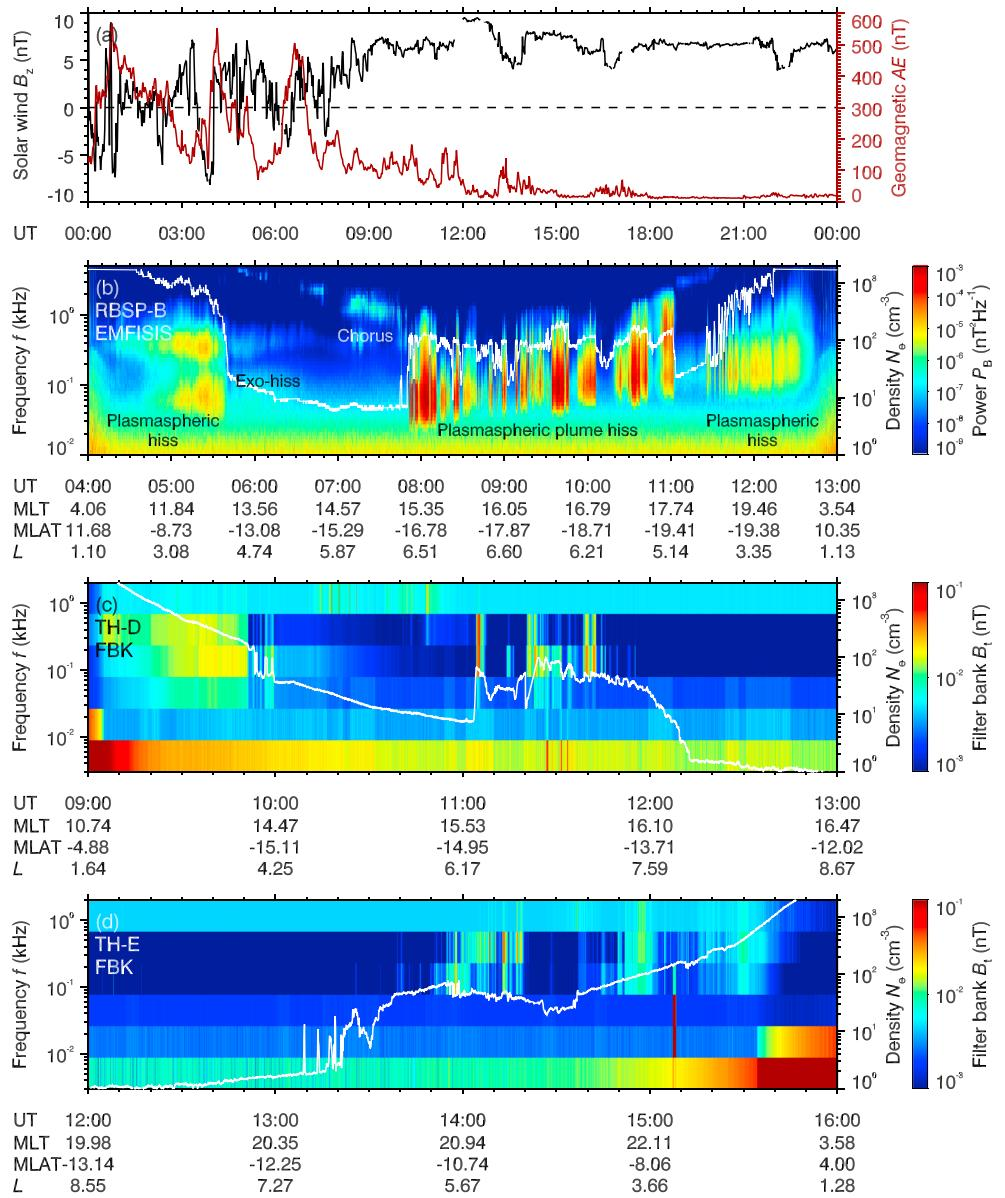
**Figure 1.** An overview of the large-amplitude hiss event on 1 December 2013: (a) solar wind magnetic field  $B_z$  and substorm index  $AE$ ; (b) wave power spectral density  $P_B$  (color coded) and cold electron density  $N_e$  (white line) observed by RBSP-B; (c, d) wave filter bank amplitude  $B_t$  (color coded) and cold electron density  $N_e$  (white line) observed by THEMIS-D and THEMIS-E.
