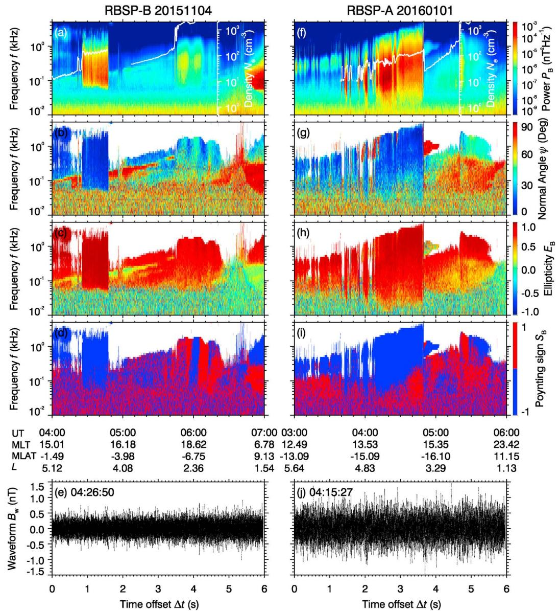
**Figure 6.** Overviews of the large-amplitude hiss events on 4 November 2015 and 1 January 2016: (a, f) wave power spectral density  $P_B$ ; (b, g) wave normal angle  $\psi$ ; (c, h) wave ellipticity  $E_B$ ; (d, i) sign of the parallel component of wave Poynting flux  $S_B$  (positive for parallel flowing and negative for antiparallel flowing); and (e, j) waveform burst  $B_w$  of plasmaspheric plume hiss.
