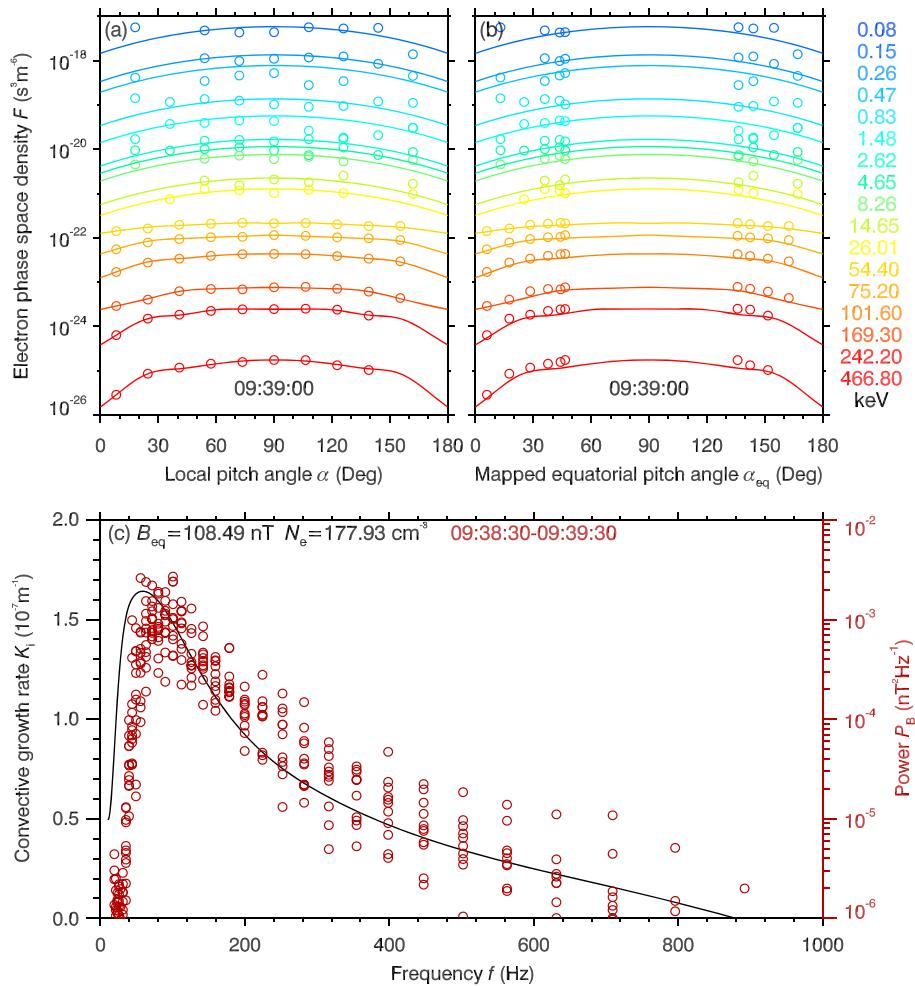
**Figure 4.** Whistler-wave instability for RBSP-B around 09:39 UT: (a) local and (b) equatorial pitch angle distributions (circles for data and solid lines for model); (c) dependence of wave convective growth rate  $K_i$  (solid line) and power spectral density  $P_B$  (circles) on frequency  $f$ .
