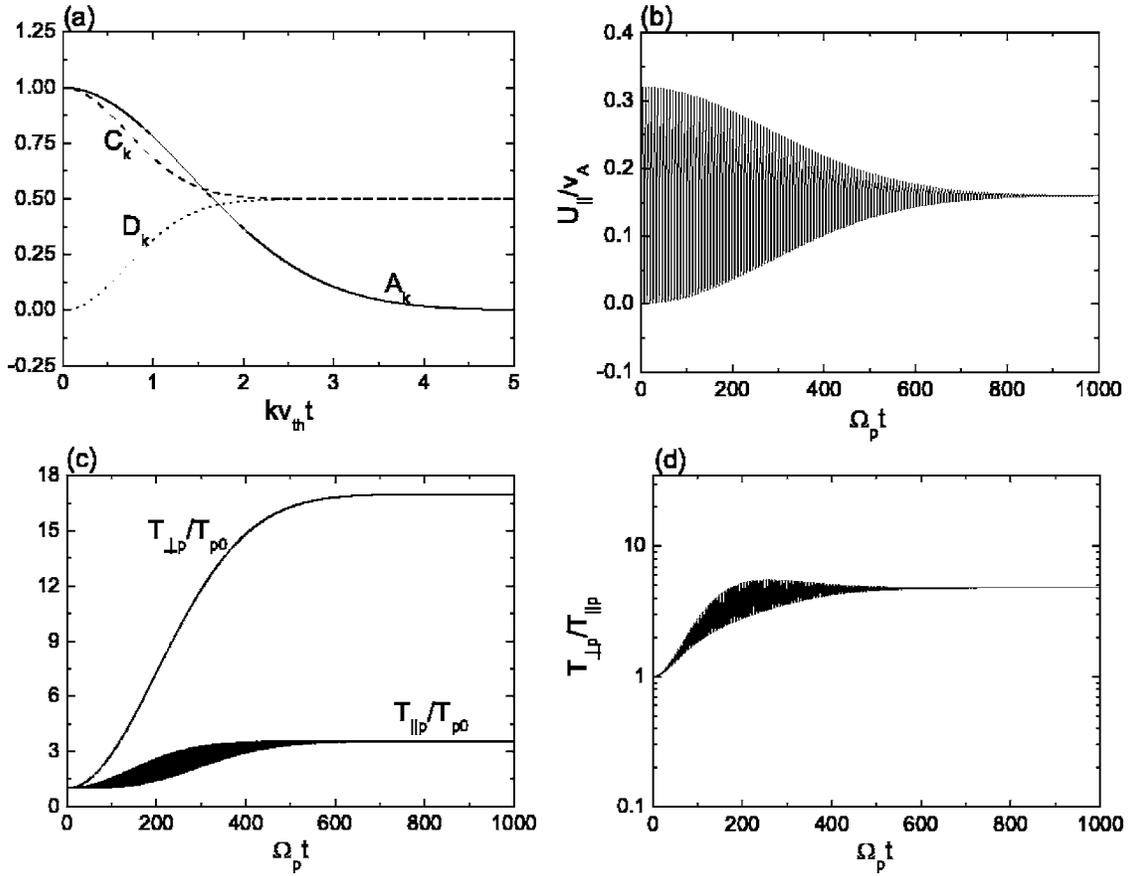
FIG. 1. The time evolution of (a)  $A_k$ ,  $C_k$ , and  $D_k$ ; (b) the average parallel velocity  $U_{\parallel}/v_A$ ; (c) the perpendicular temperature  $T_{\perp p}/T_{p0}$  and parallel temperature  $T_{\parallel p}/T_{p0}$ ; and (d) the temperature anisotropy  $T_{\perp p}/T_{\parallel p}$ . The results are based on an analytical model.
