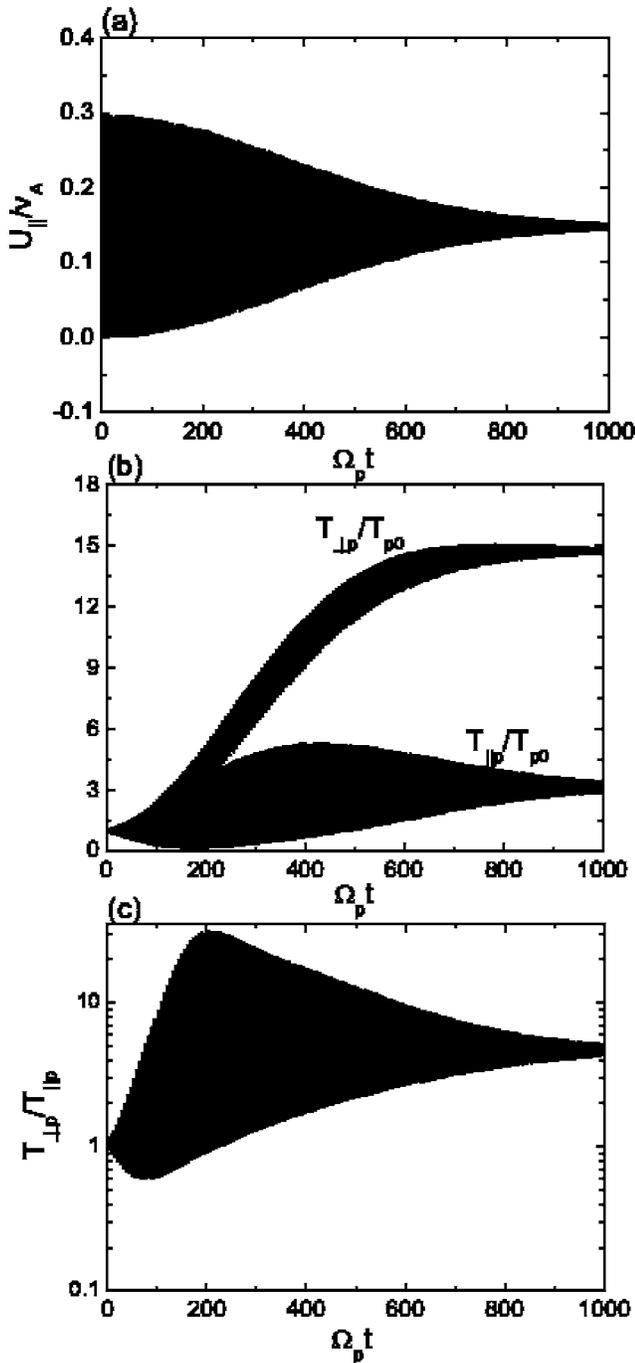
FIG. 2. The time evolution of (a) the average parallel velocity  $U_{\parallel}/v_A$ , (b) the perpendicular temperature  $T_{\perp p}/T_{p0}$  and parallel temperature  $T_{\parallel p}/T_{p0}$ , and (c) the temperature anisotropy  $T_{\perp p}/T_{\parallel p}$ . The results are based on test particle calculations.
