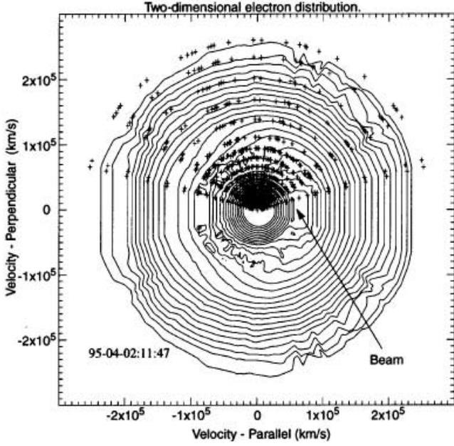
FIG. 1.—Contour plot of the two-dimensional electron distribution, which includes the beam and background electrons. The contours represent logarithmically spaced levels. The plus signs are the center velocities of the EESAH and SST Foil detectors. The beam is at  $\sim 6 \times 10^4$  km s $^{-1}$ . (After Ergun et al. 1998.)
