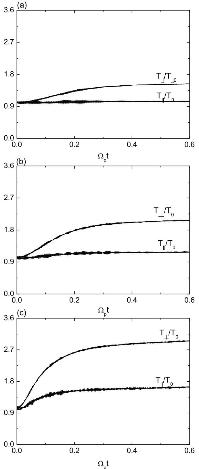
FIG. 3.—Time evolution of the effective parallel and perpendicular temperature  $T_{\parallel}/T_0$  and  $T_{\perp}/T_0$ , respectively, for three cases: (a)  $\delta B_w^2/B_0^2 = 0.064$ , (b)  $\delta B_w^2/B_0^2 = 0.142$ , and (c)  $\delta B_w^2/B_0^2 = 0.319$ . The results are based on test particle calculations.
