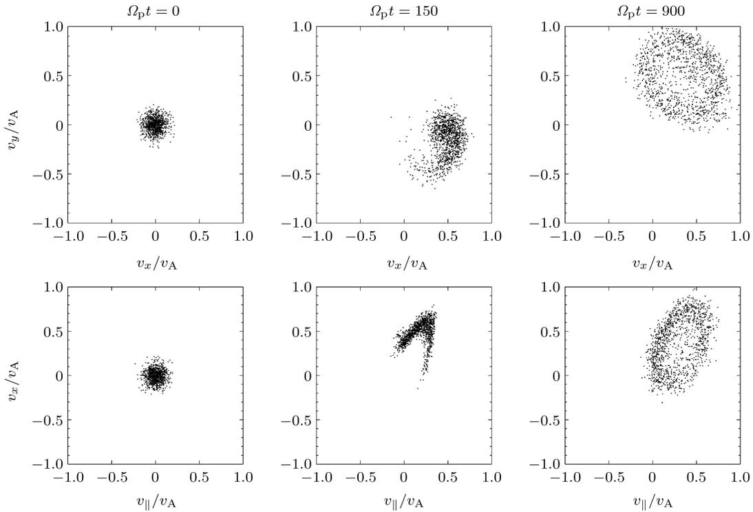
**Fig.3.** The evolution of velocity distribution of protons in a small region between  $697 v_A \Omega_p^{-1}$  and  $703 v_A \Omega_p^{-1}$ .
