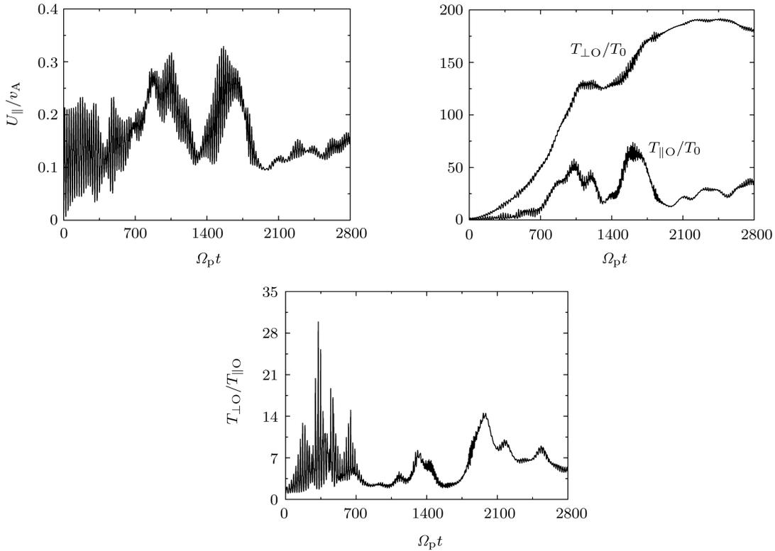
**Fig.5.** The time evolution of the average parallel velocity  $U_{\parallel}/v_A$ , the parallel temperature  $T_{\parallel O}/T_0$ , the perpendicular temperature  $T_{\perp O}/T_0$ , and the temperature anisotropy  $T_{\perp O}/T_{\parallel O}$  for  $O^{5+}$ .
