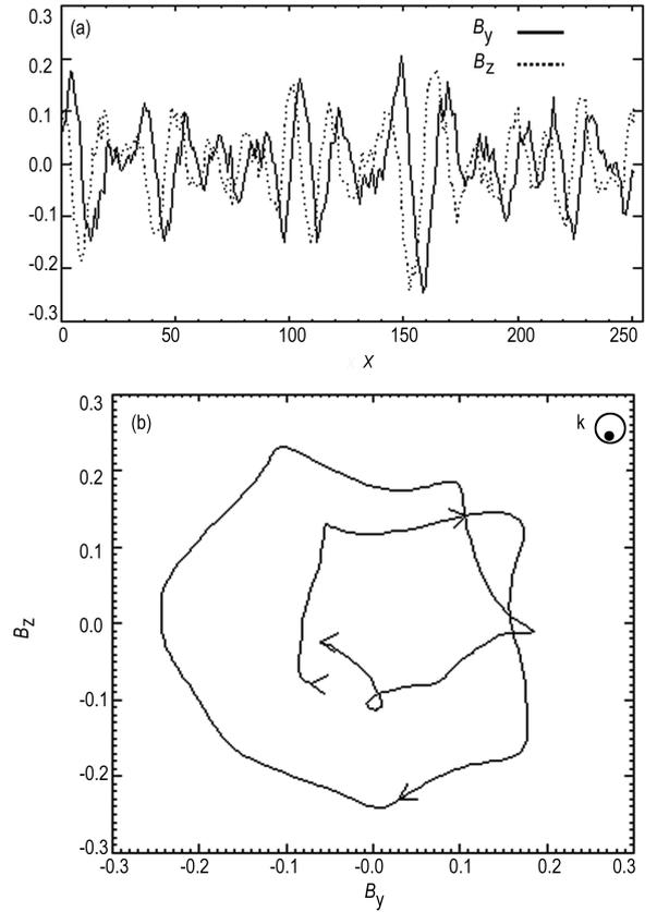
**Fig.7** (a) Spatial distribution of the magnetic fields at  $\Omega_p t = 80$ . (b) Hodograph of the magnetic fields at  $nx = 160$  and with the time interval  $\Omega_p t$  from 62 to 102
