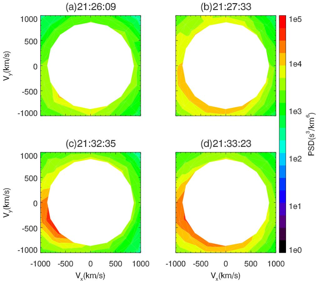
**Figure 5.** Projection of ion distributions in the velocity space measured by CIS/CODIF in unit of phase space density ( $\text{s}^3 \text{km}^{-6}$ ) observed by C1 at the time (a) 21:26:09 UT, (b) 21:27:33 UT, (c) 21:32:35 UT, and (d) 21:33:23 UT. Only the distributions of superthermal ions with the energy greater than 3 keV are plotted.
