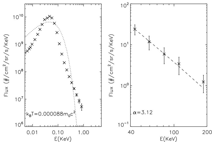
**Figure 3.** The electron differential fluxes as a function of the electron kinetic energy during the interval 0931–0934 UT for (left) low energy and (right) high energy. The dashed line is fitted by the nonlinear least squares method with LMFIT function in the program Interactive Data Language, which utilizes Levenberg-Marquardt algorithm. The differential fluxes at lower and higher energies are modeled by Maxwellian and power law distributions. The error bars are also plotted.
