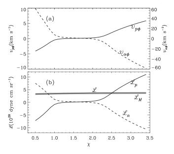
Fig. 6.—Values of several parameters at 1 AU as a function of parameter  $\chi$ : (a) azimuthal speeds of protons  $v_{p\phi}$  and alpha particles  $v_{\alpha\phi}$ , and (b) specific angular momentum fluxes carried by the proton fluid  $L_p$ , the alpha-particle fluid  $L_\alpha$ , and magnetic stresses  $L_M$ . The total flux L is also given.
